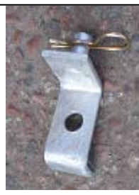
5. Corner plate Z to tension tube.
