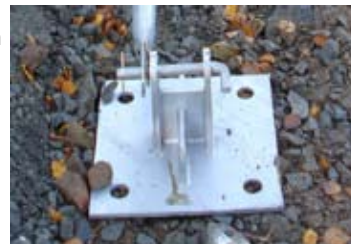
2. Ground plate, foot pin, hairpin spring and tension tube.
